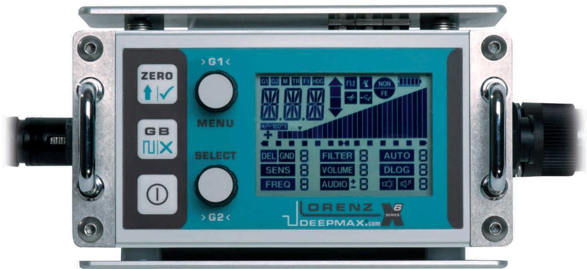
The front panel controls of the two detectors X5 and X6 are the same, namely three push buttons with **ZERO**, **GB** Ground Balance, and **POWER** function and two incremental encoders with push button for **MENU** and **SELECT**. The X6 offers an additional data logger function which can also be set by means of **ZERO** and **GB** controls when the data logger function is turned on.
